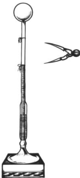
Figure 1.2 An early air thermometer or thermoscope. The thermoscope consists of a glass bulb with a long capillary attached immersed in water or oil. With an increase in the temperature, the air in the bulb expands lowering the fluid level. The scale was marked using two fixed points as indicated by the pieces of string, and interpolated using a pair of dividers to measure intermediate steps or degrees
