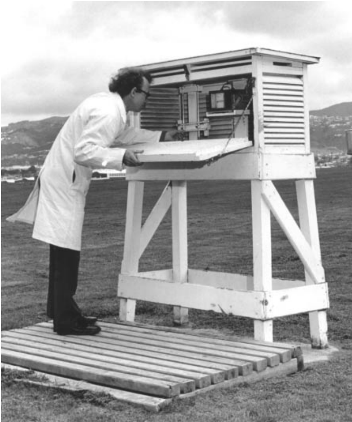
Figure 1.7 A large double-louvered thermometer screen of the Stevenson type. The screen contains a thermograph, wet bulb and dry bulb thermometers, and maximum and minimum thermometers. Note that the screen is located clear of buildings and well off the ground
