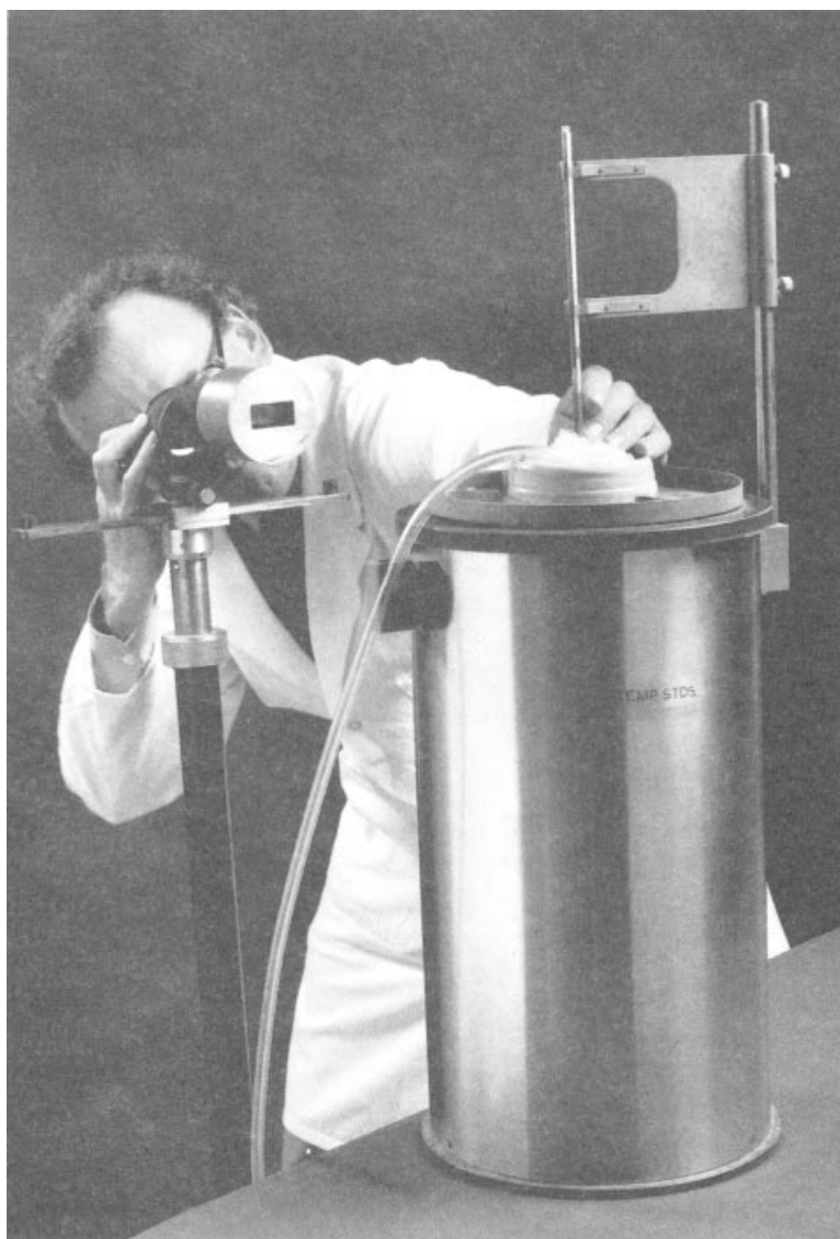
Figure 7.10 A simple monocular telescope with a close-up lens being used to read the ice point on a mercury-in-glass thermometer. The telescope is on a heavy stand to free the user's hands, and its height is set on the same level as the top of the mercury to avoid parallax errors. The distance is about an arm's length, allowing the user to adjust the thermometer for position, clear any fogging or obstacle away from the scale and to be able to tap the thermometer just before the reading is made
