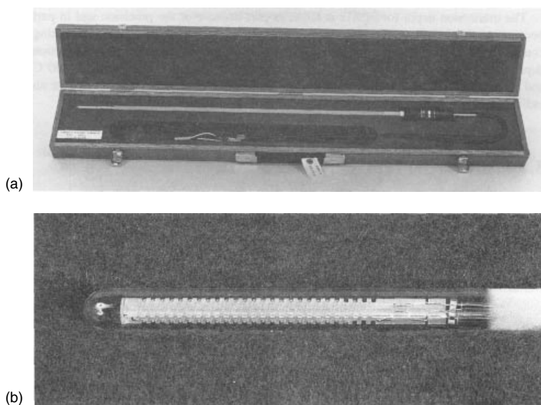
Figure 3.13 A long-stem SPRT made to ITS-90 requirements. The complete assembly in a carrying case is shown (top), with the tip showing details of construction of the resistance element (below)
