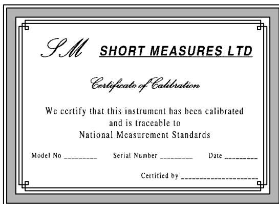
Figure 5.1 When is a calibration certificate not a calibration certificate? The type of document shown here provides no measure of the instrument’s relationship to ITS-90, or uncertainty in readings; indeed it does not mention temperature at all. It is a manufacturer’s warranty indicating that the manufacturer has made the appropriate adjustments, and not a calibration certificate
