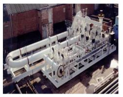
This concept has been refined to allow the design and manufacture of standardised measuring devices called 'pipe provers'. These devices are used extensively to measure all types of high value fluid from LPG to high viscosity crude oil. They are produced in all sizes from 50 mm to 1250 mm (2-48 inches).
