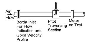
To use this method, the installation and the positioning of the sensor has to be carried out accurately. The cross sectional area of the duct has to be known, and an ideal flow profile present to allow the calculation of volume flow from point velocity. Insertion meters can be used by inserting them into an existing duct or pipe and this can be done without stopping the process. This will allow an installed meter to be verified in-situ.
