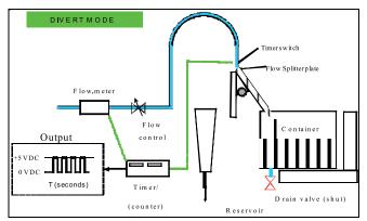
the potential for a change in flowrate during a test. The diverter mechanism is operated as quickly as possible to reduce 'timing errors' to a minimum. With a well designed diverter, test filling times down to 30 seconds can be achieved.
