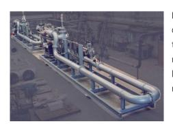
Located at the end of the prover is the sphere handling valve arrangement, designed to hold the sphere. At the start of a test the sphere is launched into the flow and carried round the loop captured and returned to the launch position ready for another run. The design of the valve is critical, and must not only be leak-tight but must have mechanisms to prove it is leak-tight. The valve also normally allows a means to remove the sphere for inspection.
