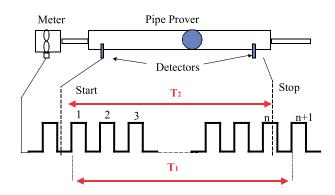
To estimate the fraction of a pulse lost or gained at the start and finish of a pass, the whole number of pulses are first counted. This total is multiplied by the interpolation factor. This is the ratio of the time between the switches, and the time between the first pulse after the start switch and the first pulse after the stop switch.
