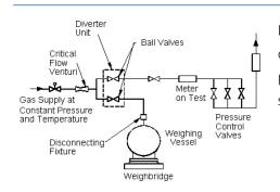
Due to gas compressibility effects, it is more difficult to maintain a closely controlled flowrate than it is for liquid flow systems. As pressure changes, potentially large changes in temperature can occur making it difficult to obtain stable conditions.
